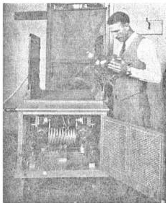
Fig. 160 Front View Short-Wave Oscillator, Oscillator Compartment Open Showing Vacuum Tubes and Main Inductance.
