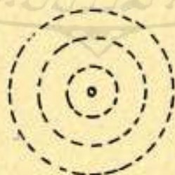
Equipotential surfaces round an isolated positively charged particle.
