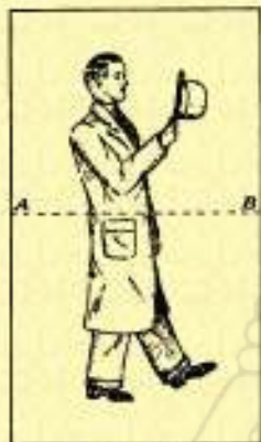
FIG. 33.—Scanning a subject of this kind produces a single pulse per line for approximately one-third of each frame.
