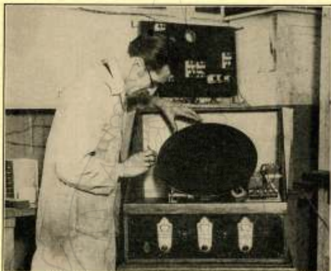
FIG. 38.—One of the first complete television reproducers offered by the Pilot Electric Company in 1929. A magnetic clutch was intended to maintain synchrony.
