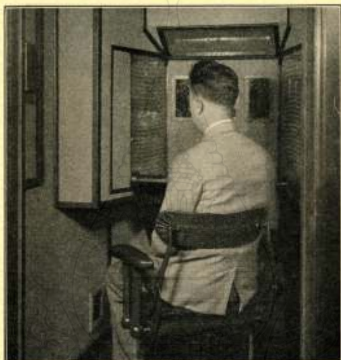
FIG. 15.—By the addition of two caesium-oxygen cells on either side and a deep-red scanning beam, much greater naturalness in shading was secured subsequent to the public two-way wire television demonstration.
