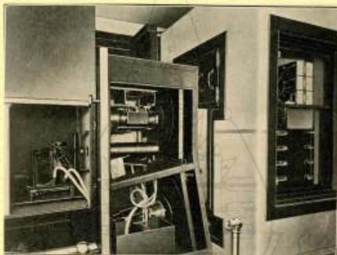
FIG. 14.—The three major units of the apparatus used in the two-way wire television demonstration. The terminals of the photoelectric pick-up system are in the unit at the right; the scanning discs for pick-up and reproduction at the center and the arc light for scanning are at the left.
