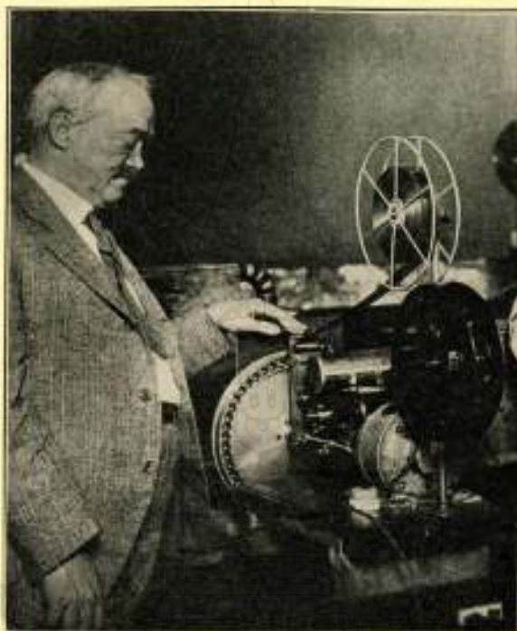
FIG. 21.—Dr. C. Francis Jenkins and his motion-picture lens scanning device.
