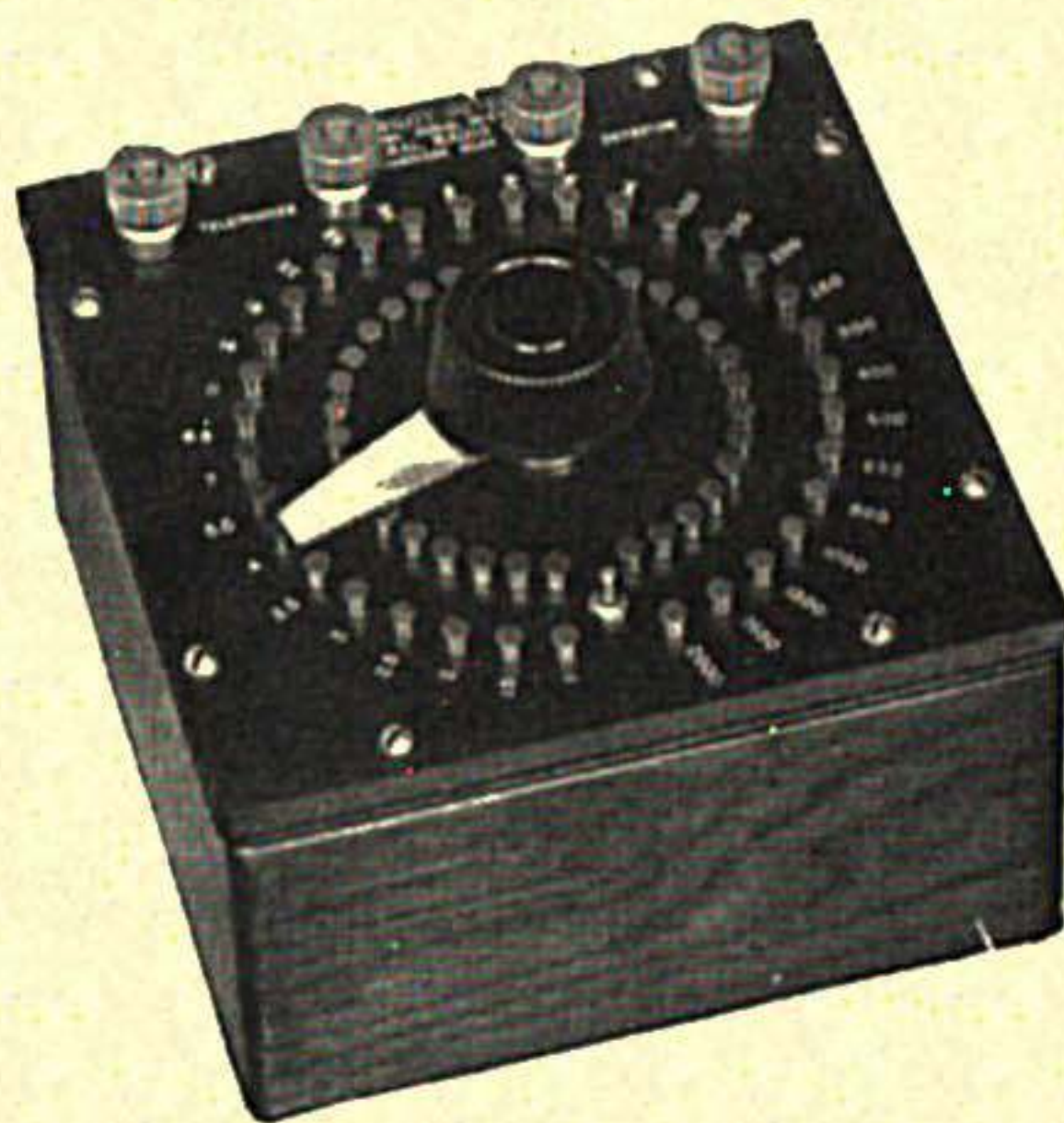
Fig. 193. General Radio Type 164 Audibility Meter
