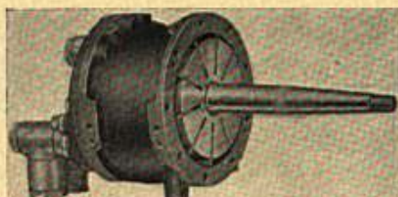
Fig. 8. SHOWING ECCENTRICALLY-PLACED ROTOR AND SLIDING VANES OF WINDMILL-DRIVEN COMPRESSOR
