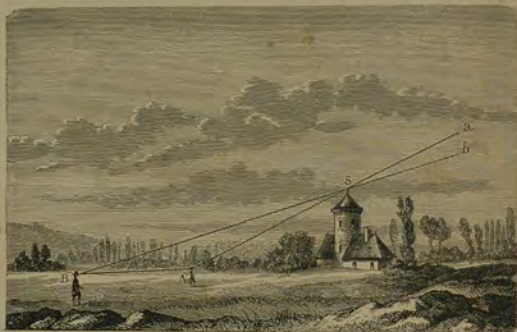
Fig. 185.—Apparent variation in the height of a tower at different distances.
