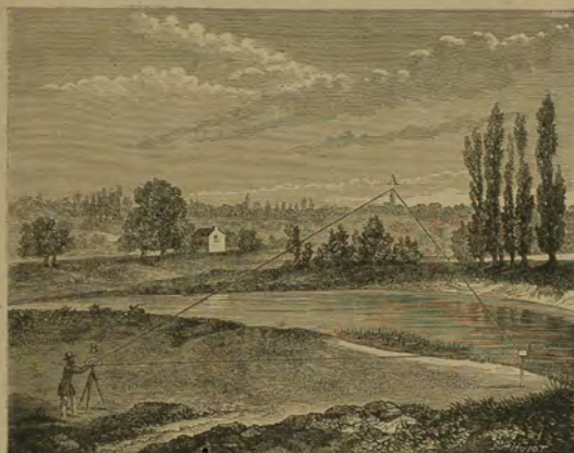
Fig. 131.—Measure of the distance of an inaccessible object.
