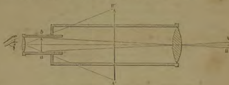
Fig. 186.—Theoretical Section of the Astronomical Telescope.
