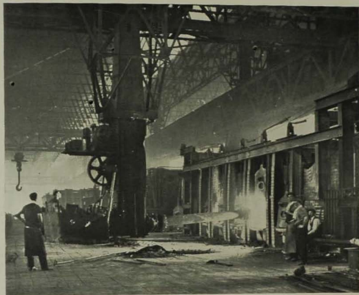
FIG. 46.—Charging Steel Furnace by means of Electric Crane suspended from overhead rail.
