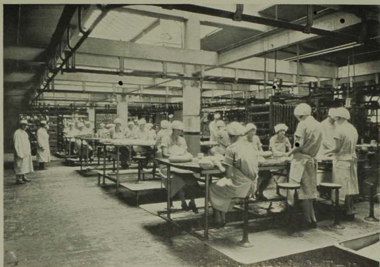
FIG. 53.—Sausage Stuffing Tables made with Monel Metal. (Messrs. John Morrell & Co., Ottumwa, Iowa.)
