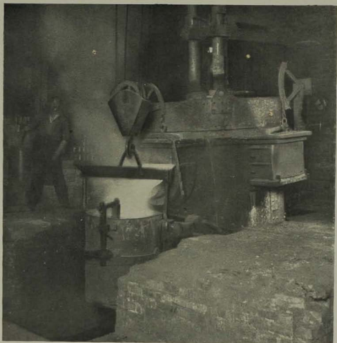
FIG. 47.—Hérault Arc Furnace. Pouring molten "Cronite" (a heat-resisting Chromium-Nickel Steel) to the Ladle at the Works of Messrs. Cronite Foundry Co., Ltd., Tottenham. ( Courtesy, Messrs. The Mond Nickel Co., Ltd., London. )
